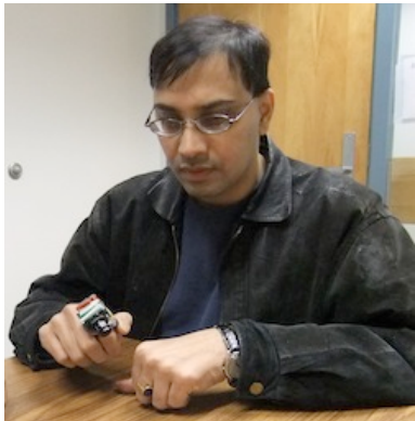
Figure 2: A blind user wearing EyeRing System. We are in the stages of developing a more slick design, which will have a center of gravity closer to the finger and overall smaller size.
